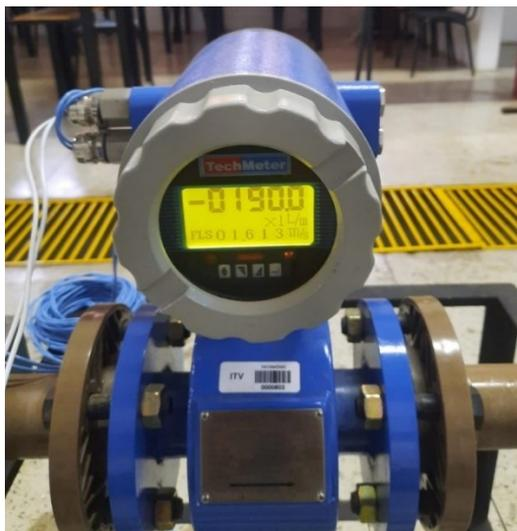
Figura 10 – Fluxômetro Techmeter HHD50K1C1E2F1T1P2D2.
