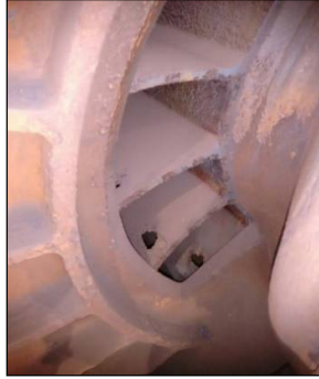
Fig.6 – Punctual holes caused by cavitation in the pallets of a LRVP in the Pelletizing unit studied
